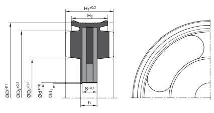
For surface finish, lead in chamfer and other installation dimensions see "General installation guidelines".
